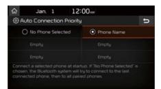
When the engine is running, the selected Bluetooth device is automatically connected. If you fail to connect the selected device, the previously-connected device is automatically connected, and if it also fails, then it tries to connect all paired devices sequentially.
