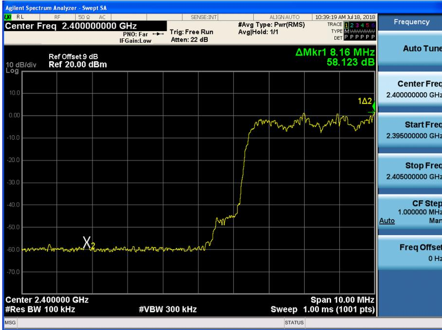
Test Plots with hopping (8DPSK)
