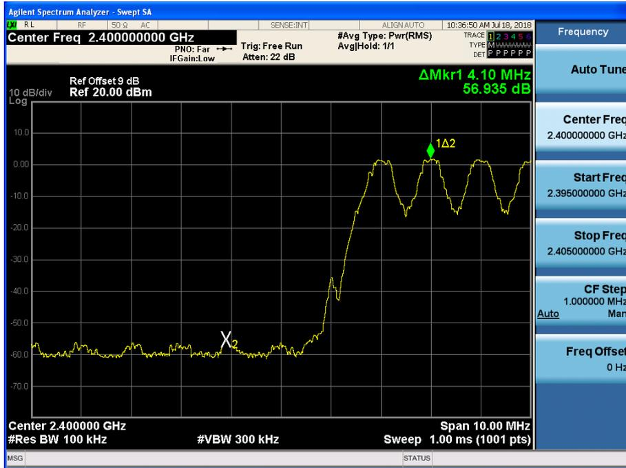
Test Plots with hopping (GFSK)
