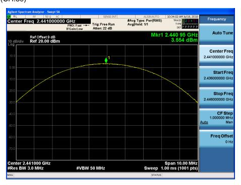
Test Plots (8DPSK) Peak Power (CH.78)
