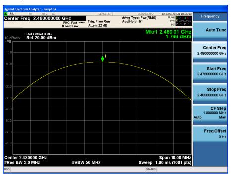
Test Plots (8DPSK) Peak Power (CH.0)
