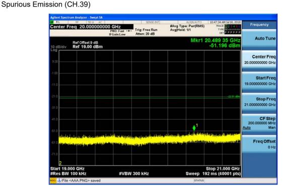
Test Plots (8DPSK)- 21 GHz - 23 GHz Spurious Emission (CH.39)
