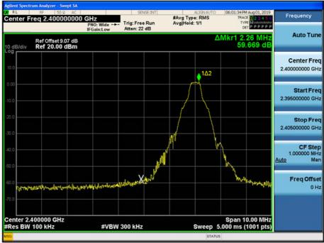
Test Plots without hopping (GFSK) Band Edges (CH.78)
