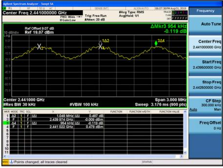
Test Plots (8DPSK) Channel Separation
