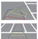
If an object comes too close to your vehicle as you are parking the vehicle, a warning beep will sound. To prevent an accident that might result if you do not hear the beep, you can set the system to decrease the volume level of any media playing automatically when you are parking the vehicle. On the Home screen, press All Menus ➤ Setup ➤ Sound ➤ Priority ➤ Proximity Warning.
