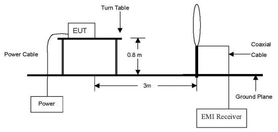
The diagram below shows the test setup that is utilized to make the measurements for emission from 30 Mb to 1 @ emissions.
