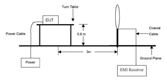
The diagram below shows the test setup that is utilized to make the measurements for emission from 30 Mb to 1 Hz.
