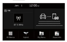
The Hybrid menu consists of three sections: Average, ECO level and Energy flow.
