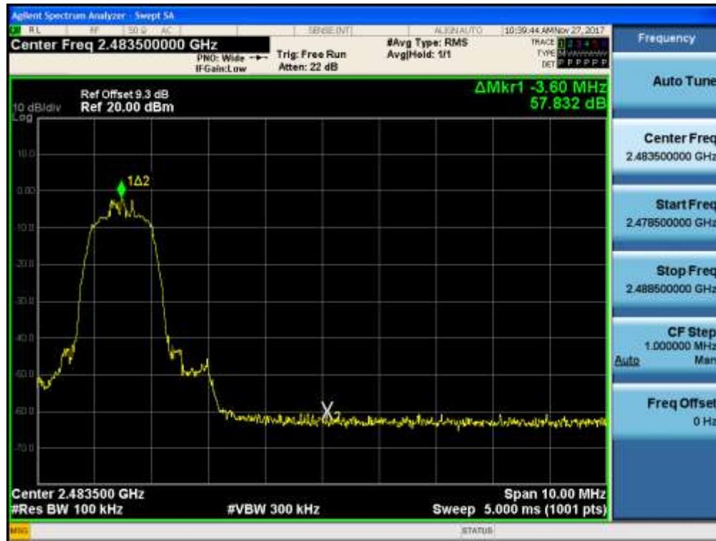
Test Plots with hopping (GFSK)
