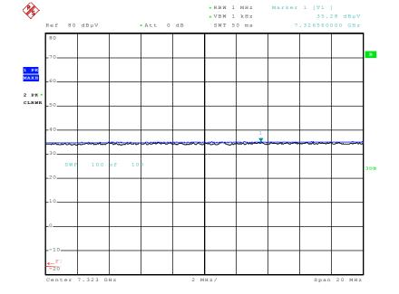
Radiated Spurious Emissions plot – Average Reading (GFSK, Ch.39 3nd Harmonic)
