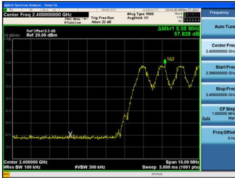
Test Plots with hopping (GFSK)
