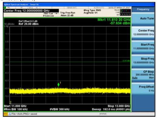
Test Plots (8DPSK)- 13 GHz – 15 GHz Spurious Emission (CH.78)
