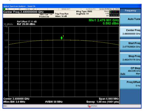
Test Plots (8DPSK) Peak Power (CH.0)
