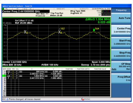
Test Plots (8DPSK) Channel Separation
