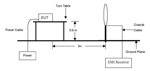
The diagram below shows the test setup that is utilized to make the measurements for emission from 30 Mb to 1 GHz.
