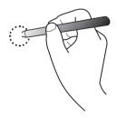
The System Reset function restores the system when it is not operating correctly. Press and hold the RESET key for a second or longer. (It is recommended that you press the RESET key using a tool, such as a pin or a clip.)
