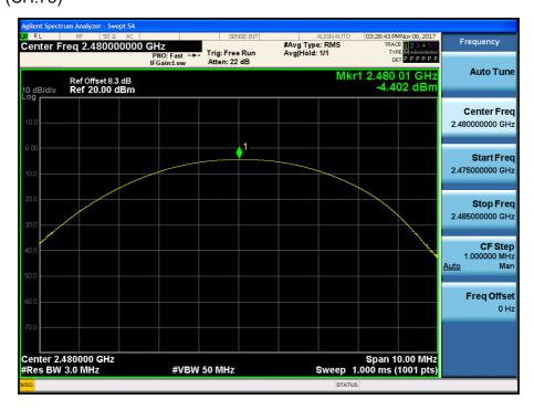
Test Plots (8DPSK) Peak Power (CH.0)
