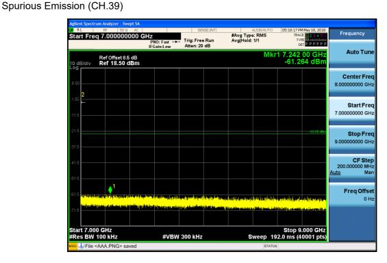
Test Plots(8DPSK)- 9 GHz - 11 GHz Spurious Emission (CH.39)
