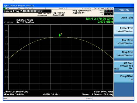
Test Plots (8DPSK) Peak Power (CH.0)
