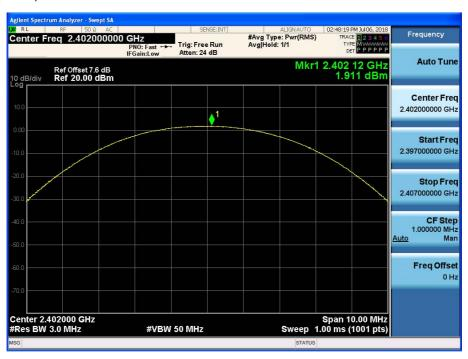
Test Plots (π/4DQPSK) Peak Power (CH.39)
