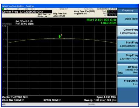
Test Plots (GFSK) Peak Power (CH.39)
