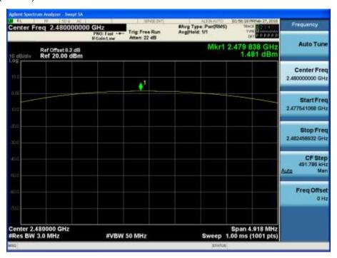
Test Plots (8DPSK) Peak Power (CH.0)
