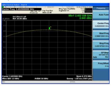
Test Plots (π/4DQPSK) Peak Power (CH.39)
