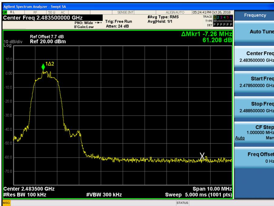
Test Plots with hopping (GFSK)
