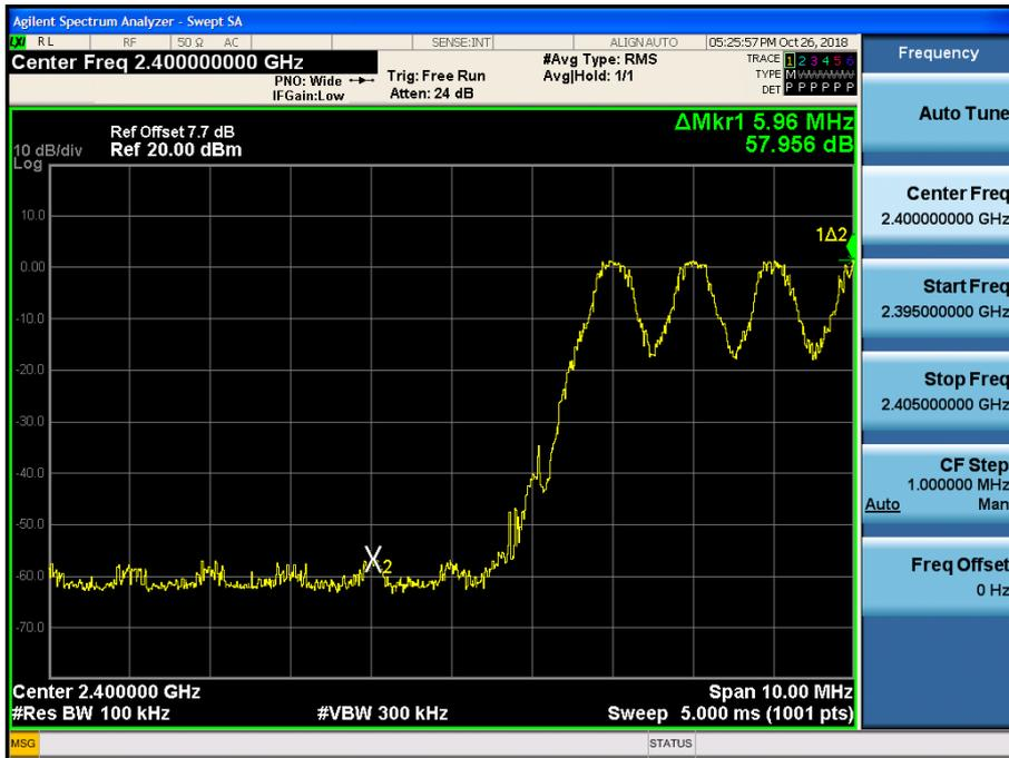
Test Plots with hopping (GFSK)
