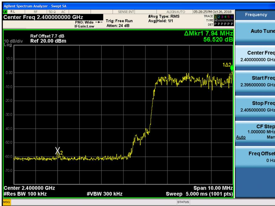
Test Plots with hopping (8DPSK)
