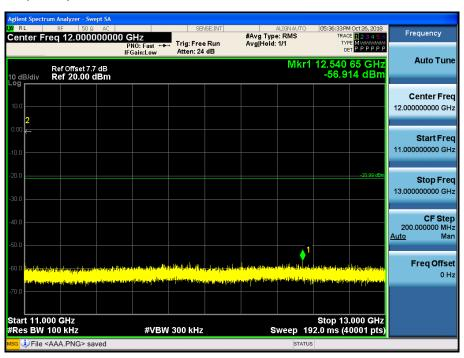
Test Plots (8DPSK)- 13 GHz – 15 GHz Spurious Emission (CH.39)
