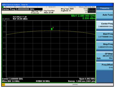
Test Plots (8DPSK) Peak Power (CH.0)
