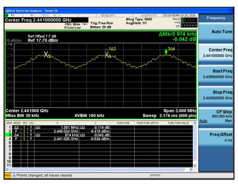
Test Plots (8DPSK) Channel Separation
