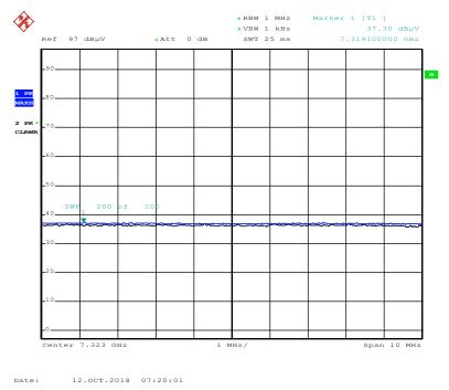
Radiated Spurious Emissions plot – Peak Reading (8DPSK), Ch.39 3rd Harmonic)
