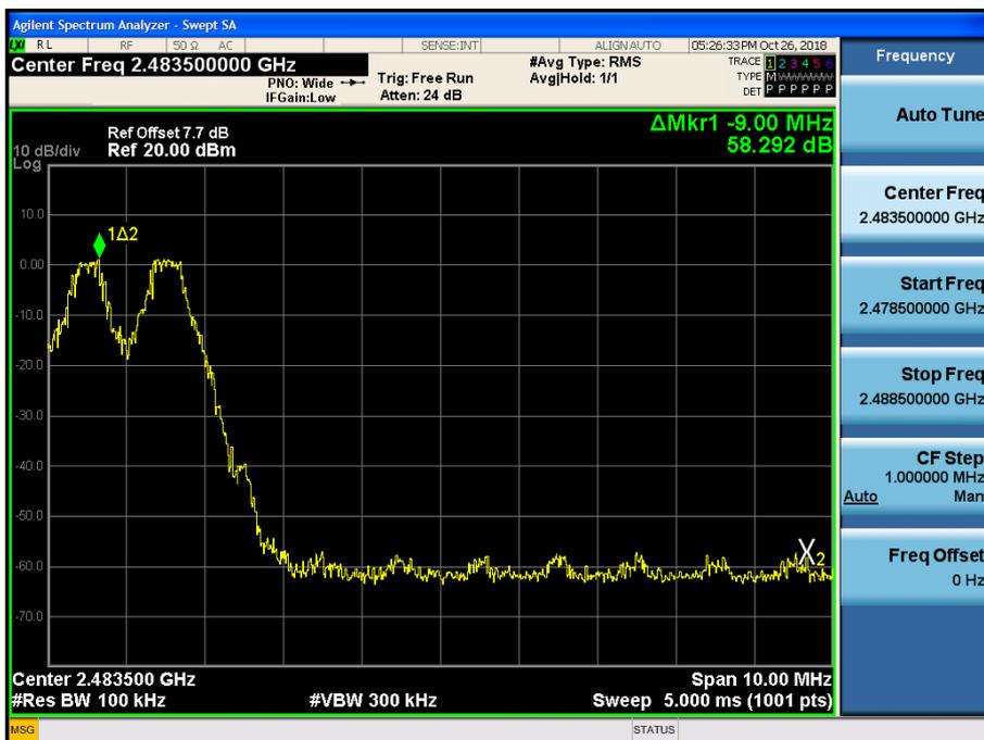
Test Plots with hopping (8DPSK)
