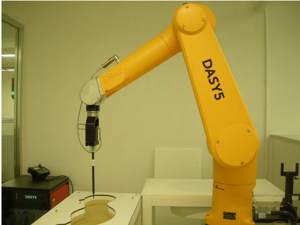
Picture B1: Specific Absorption Rate Test Layout
