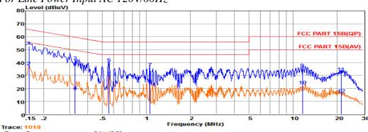
Env. Ins: EUT: M/N: Power Rating: Test Mode: Operator: Memo: Pol: 24\*/56% Smart Phone XC1003 AC 120V/60Hz TX-2402 KYLE
