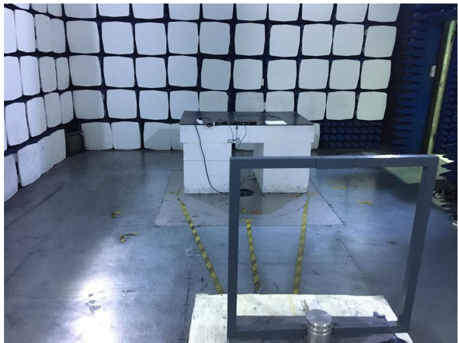
Radiation Emission Test Setup (Below 30MHz)
