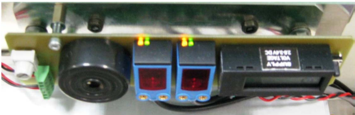
Figure 4.3: Light Barrier Orange and Green LED Lit when positioning correct (previous model)
