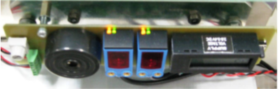
Figure 4.3: Light Barrier Orange and Green LED Lit when positioning correct (previous model)
