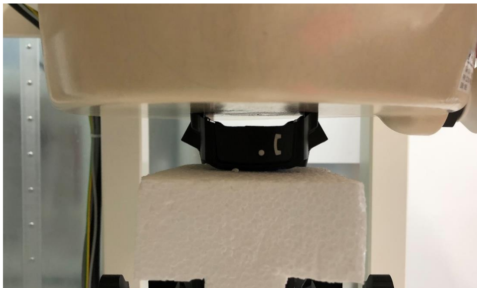
Top view of EUT against flat area of phantom with 0mm spacing
