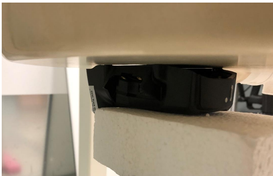
Side view of EUT against flat area of phantom with 0mm spacing
