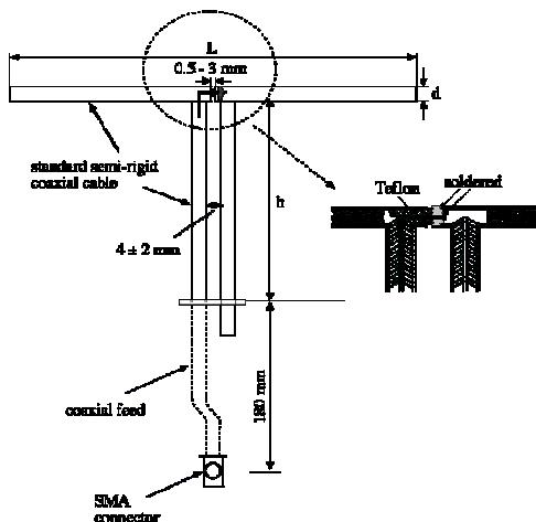
APREL Laboratories have developed high frequency dipoles based on current scientific research carried both experimentally and numerically here at the APREL Laboratories site. Mechanical and electrical parameters for the dipoles have been established using experimental and numerical techniques, and target SAR values have been established following IEC methodologies. The results of the experimental and numerical research have been published and released for peer review.
