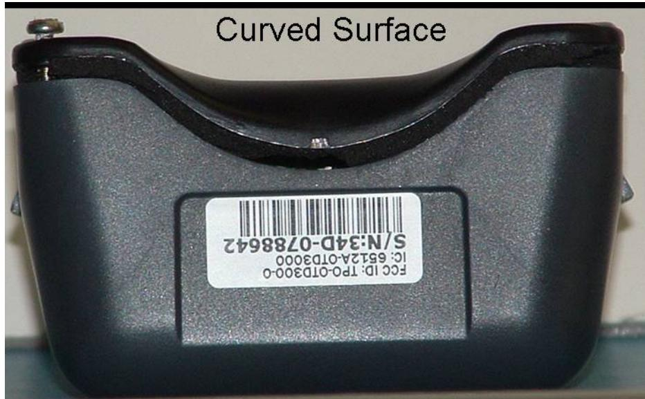
The front of the OTD has a large protrusion which is where the battery is located. This protrusion acts as a separator and would not allow for the OTD to come into touch with the user. The separation which the form of the device provides is 13mm.
