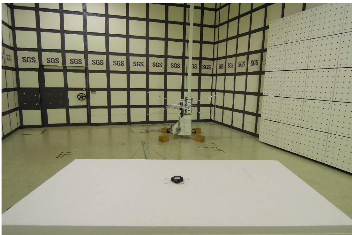
**Radiated Emission Set up Photos (E2 PLANE) (Above 1GHz)**
