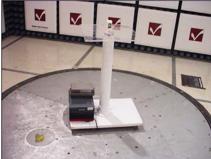
EUT setup in the test chamber View as seen by sense antenna.
