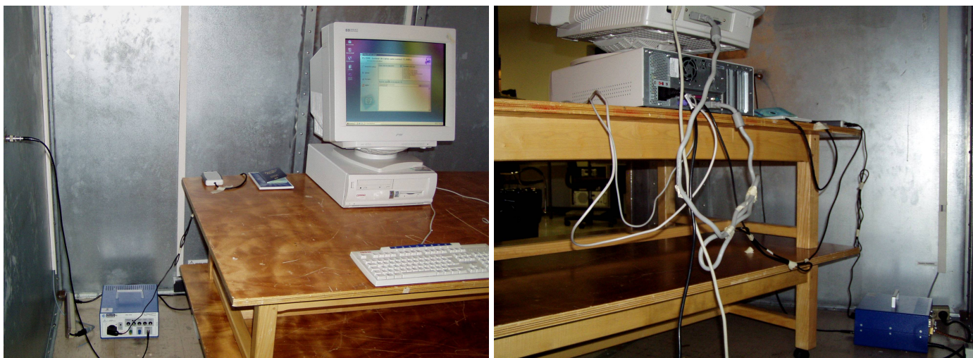
Conducted emission test setup
