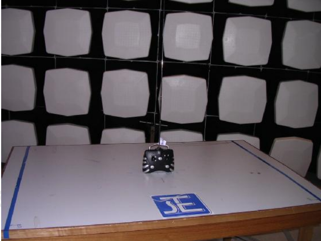
Measurement of Radiated Emission Test Set Up
