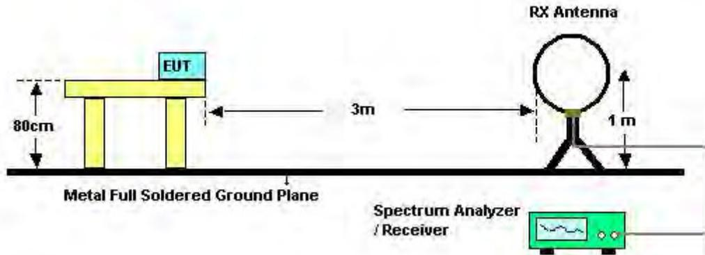
For Radiated Emissions: 30MHz~1GHz
