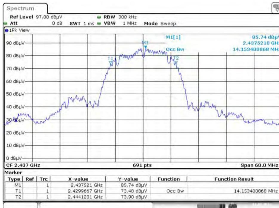
6 dB Bandwidth Plot on Configuration IEEE 802.11g / 2437 MHz / Chain 1 + Chain 2 + Chain 3 + Chain 4
