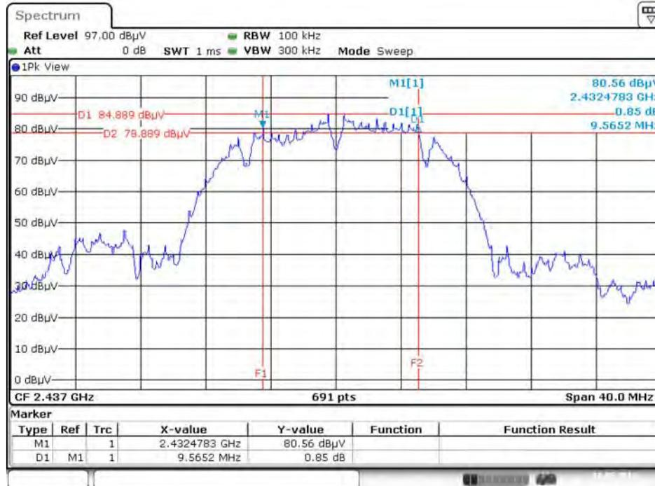
99% Occupied Bandwidth Plot on Configuration IEEE 802.11b / 2437 MHz / Chain 1 + Chain 2 + Chain 3 + Chain 4
