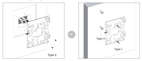
Affix the mounting bracket on to the wall using the appropriate screws from the mounting accessories included in the package
