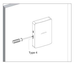
Mount the device on the bracket by aligning the two notches on the bracket with the two grooves on the rear panel of the device. Slide the device and tighten it onto the bracket with the screw provided in the package.
