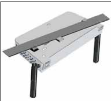
Figure 44. Initial Twisting of the Mount
