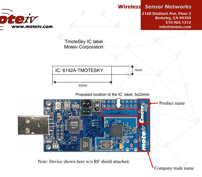
The label would take a form of a sticker permanently glued to the PCB. Note that the company trade name and the product name are already permanently fixed in the product PCB silkscreen. If the above label is not compliant, we'd propose option 2, where all the information required by the RSS-GEN section 5.2 is present on a 5x22mm label:
