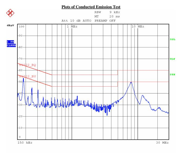
Test Model: VMP-200 Test Mode: NEUTRAL Classification: FCC Part15 Subpart B Section 15.107(g) Class B
