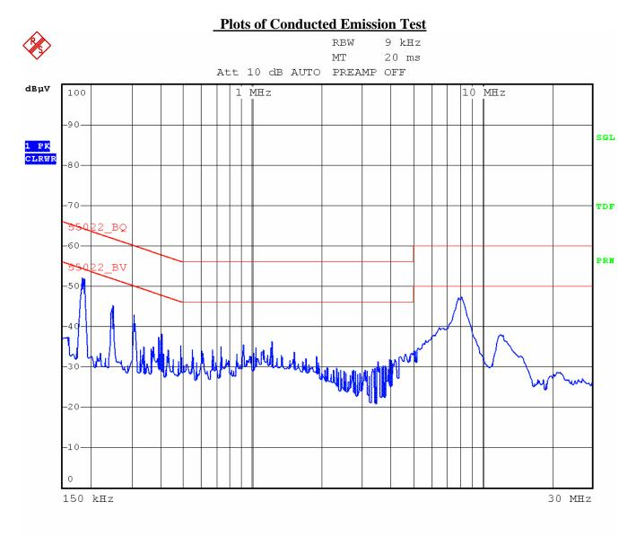
Test Model: VMP-200 Test Mode: HOT Classification: FCC Part15 Subpart B Section 15.107(g) Class B
