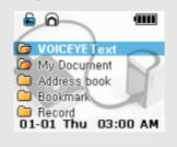
The icons for lock status, scanner connection status, and remaining battery indication are displayed in the top. In the middle, a list of folders and files are displayed. On the bottom, the current date, the day of the week and the current time are displayed. If you press the Right button after selecting a folder, the list of files and folders within the folder are displayed. If you press the Play button, the content of the selected file is shown on the display.
