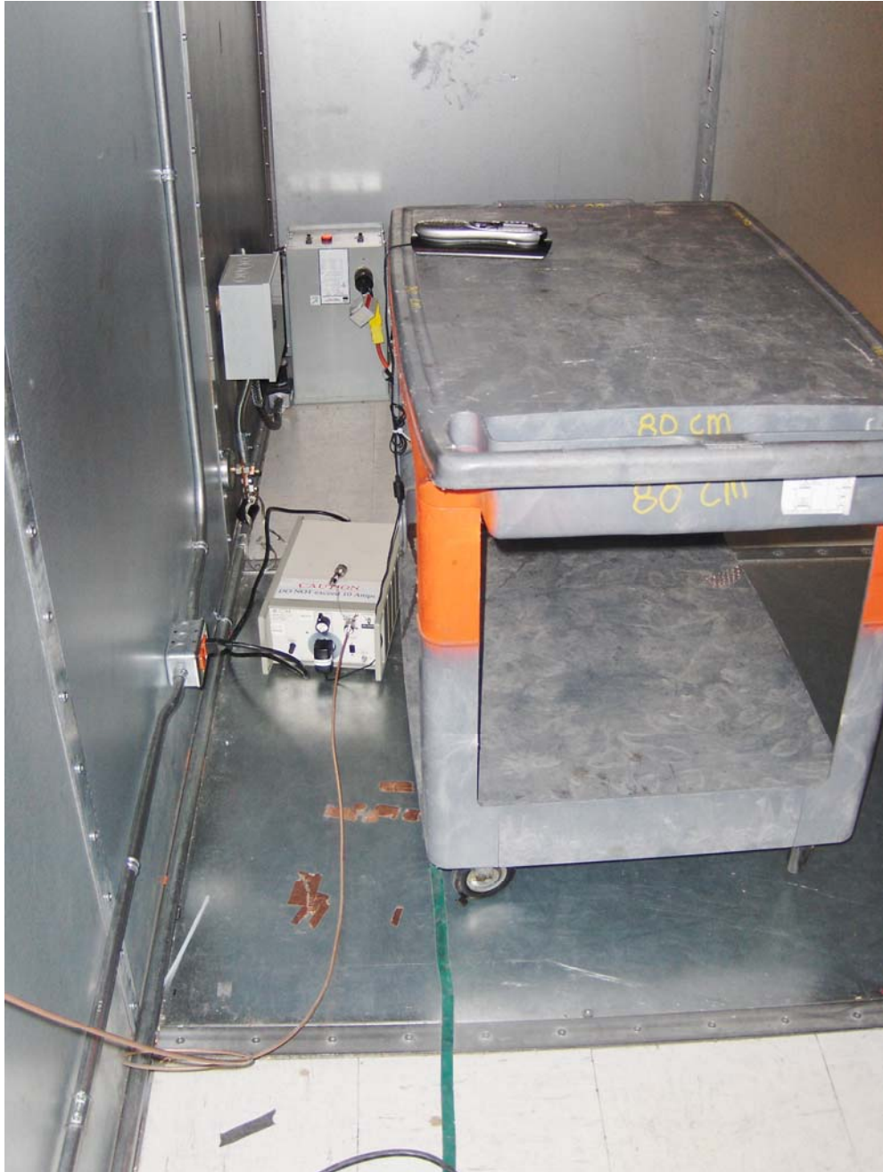
Power Line Conducted Emissions Test Configuration 1: EUT on charging cradle
