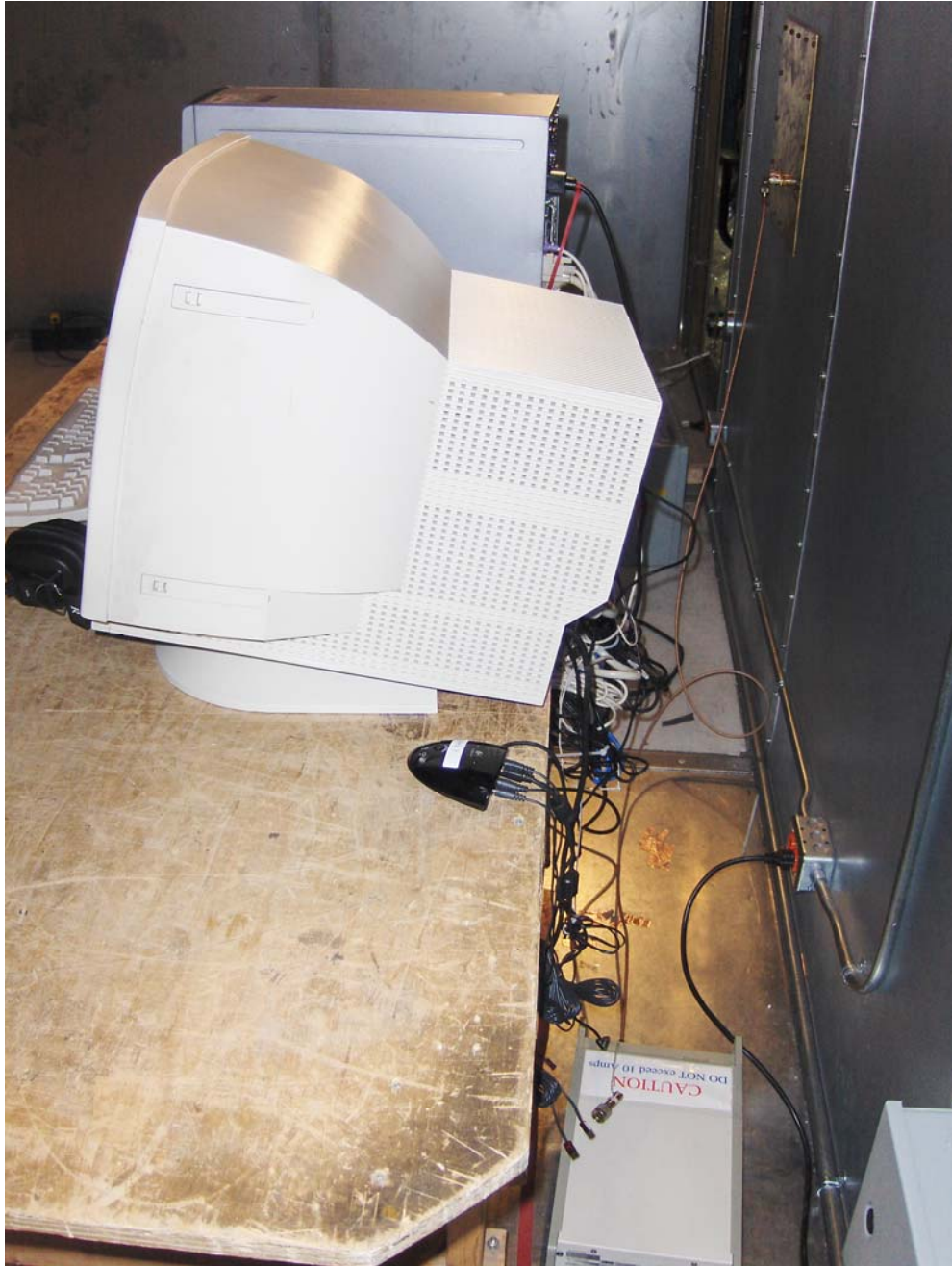
Power Line Conducted Emissions Test Configuration 2: EUT connected to PC; no power connection
