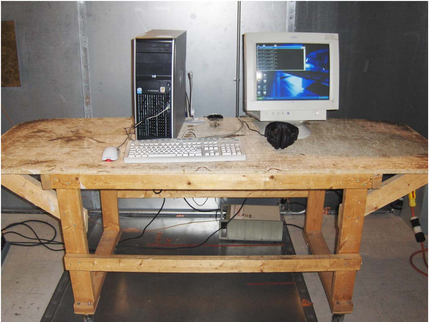
Power Line Conducted Emissions Test Configuration 2: EUT connected to PC; no power connection
