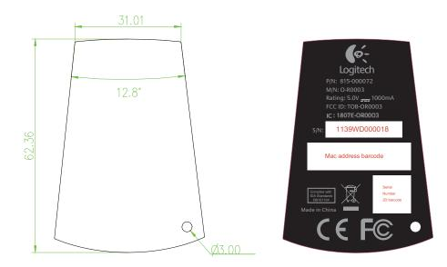
Material:FASSON Semigloss paper,80g coated art paper Thickness: 0.1mm +/-10% Adhesive: general purpose permanent, acrylic based adhesive Printing color: K80 & 877c
