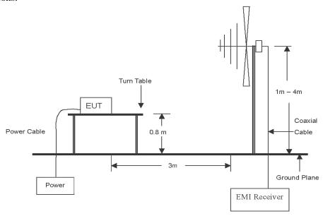
The diagram below shows the test setup that is utilized to make the measurements for emission from 1  $\,\text{GHz}\,$  to the tenth harmonic of the highest fundamental frequency or to 40  $\,\text{GHz}\,$  emissions, whichever is lower.
