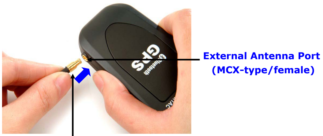
Connector of the optional External Active Antenna (MCX-type/male)
