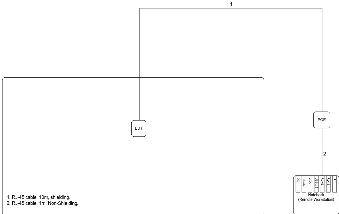
1. RJ-45 cable, 10m, shielding.
