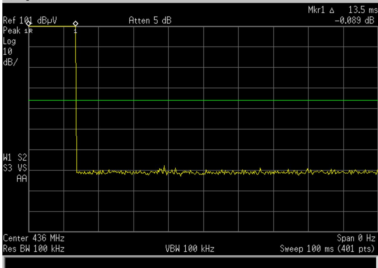
**Test Method: FCC Part 15.35, Duty Cycle Determination - 436 MHz**
