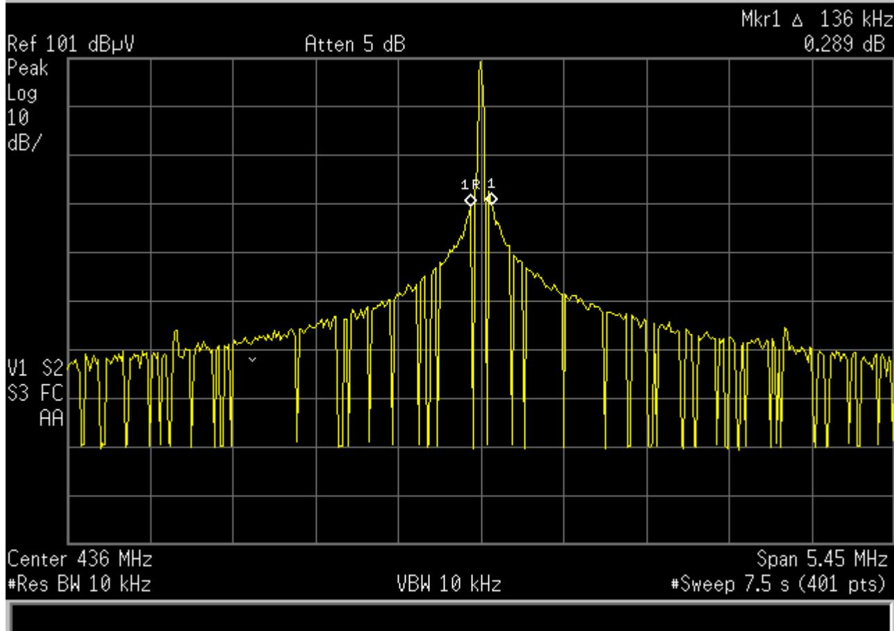
**Test Method: FCC Part 15, Subpart C, 15.231(c), Occupied Bandwidth - 436 MHz**
