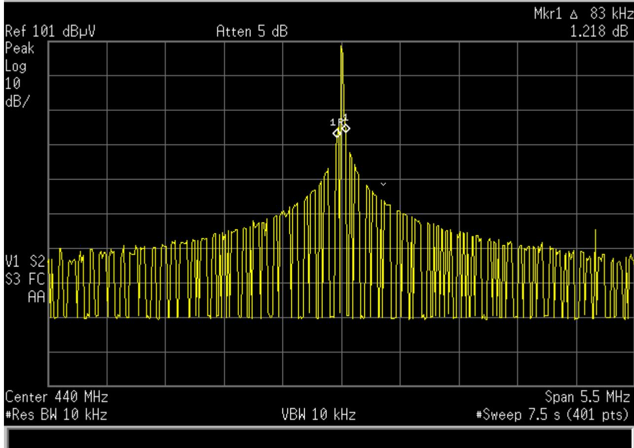
**Test Method: FCC Part 15, Subpart C, 15.231(c), Occupied Bandwidth - 440 MHz**
