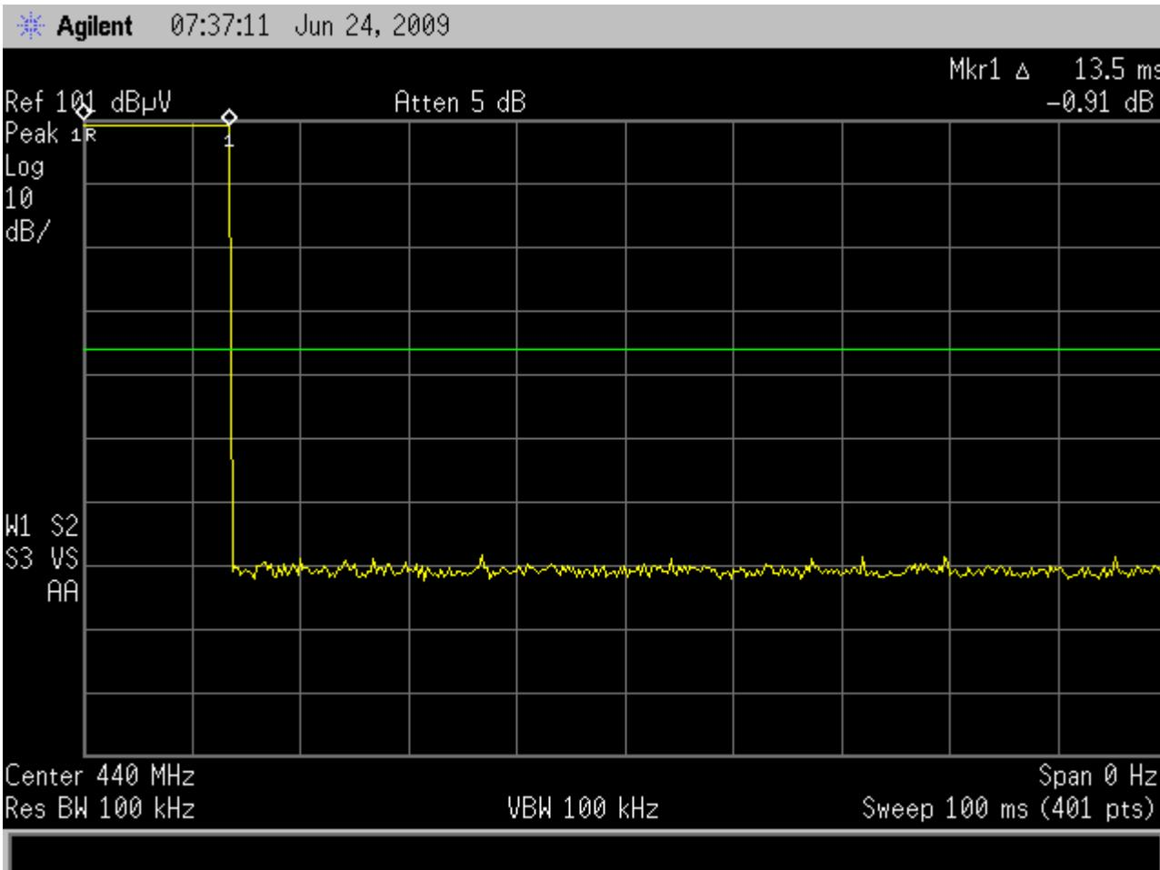
**Test Method: FCC Part 15.35, Duty Cycle Determination - 440 MHz**
