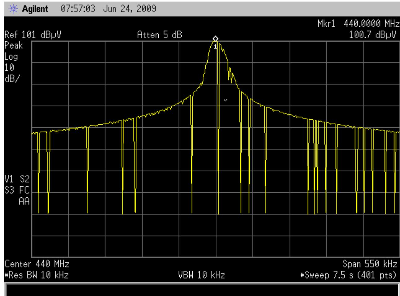
**Test Method: FCC Part 15, Subpart C, 15.231(c), Occupied Bandwidth - 440 MHz**
