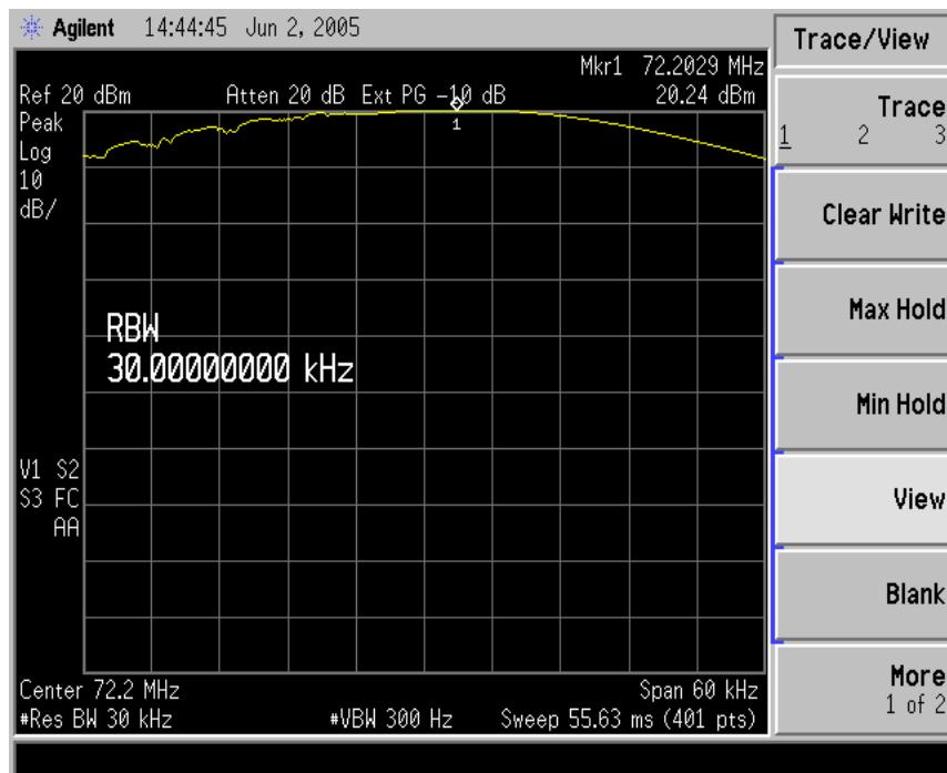
13. **Conducted Spurious Emissions: 47 CFR 2.1051**
