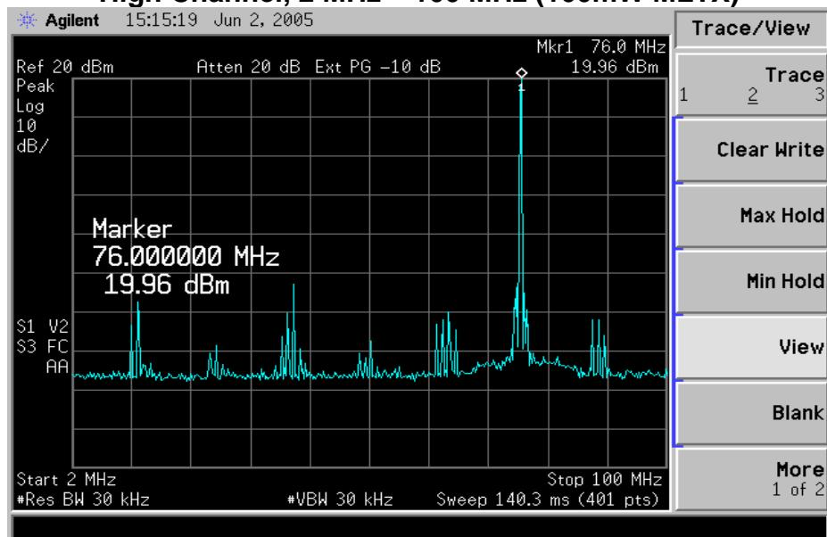
**Signature Scan of Conducted Spurious measurements**
