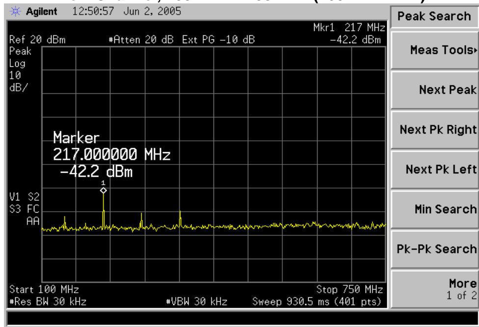
**Signature Scan of Conducted Spurious measurements**
