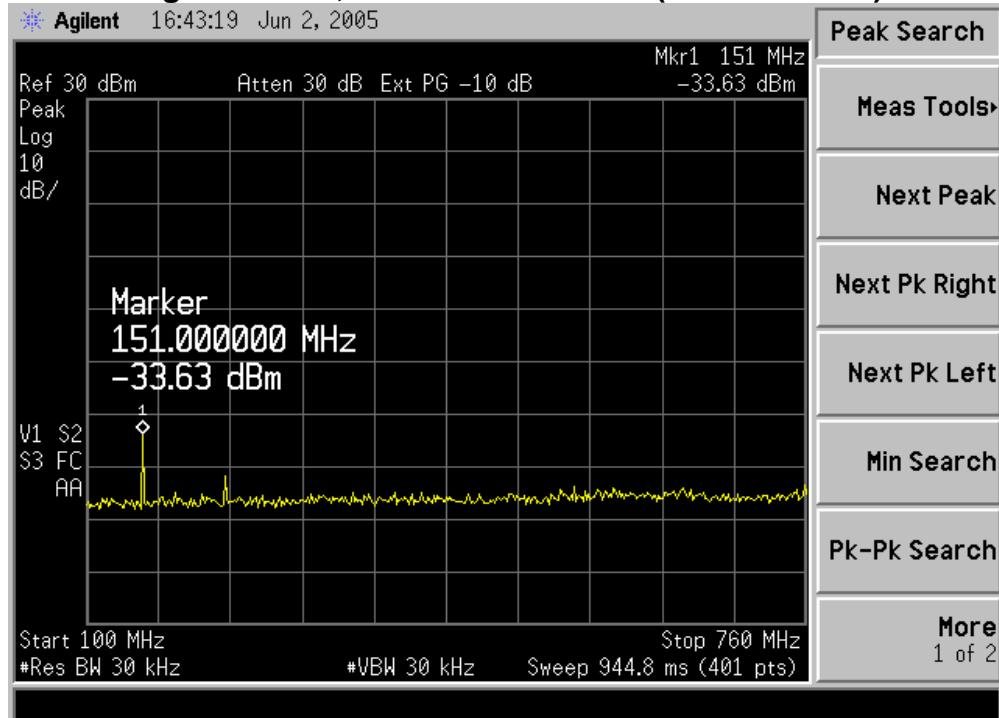
**Signature Scan of Conducted Spurious measurements
