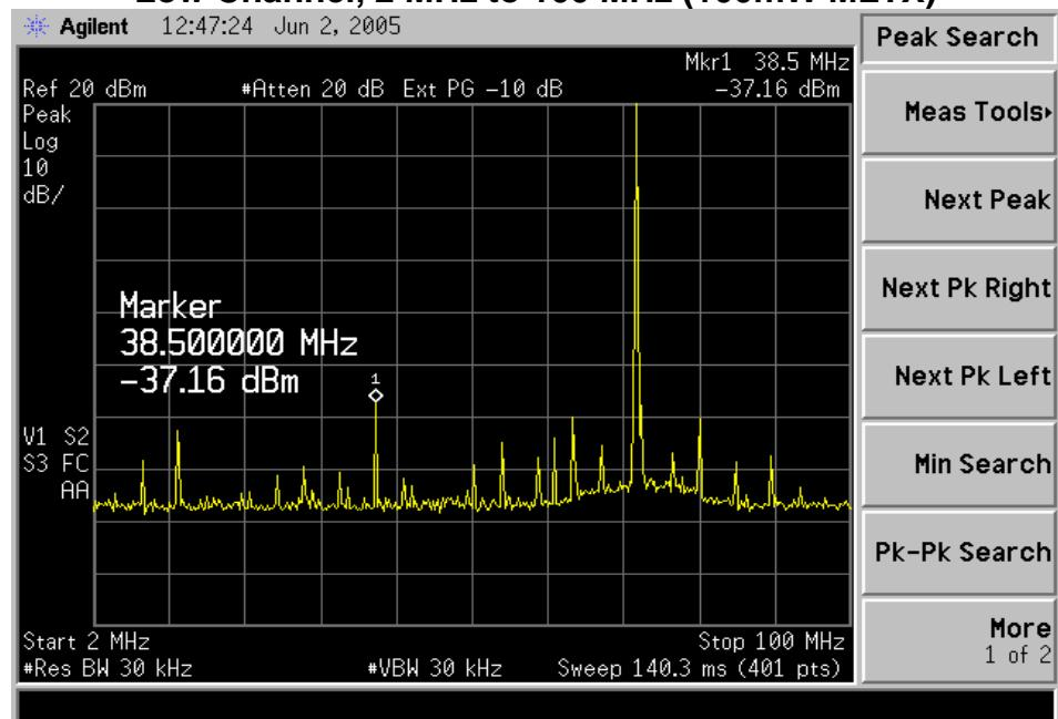
**Signature Scan of Conducted Spurious measurements
