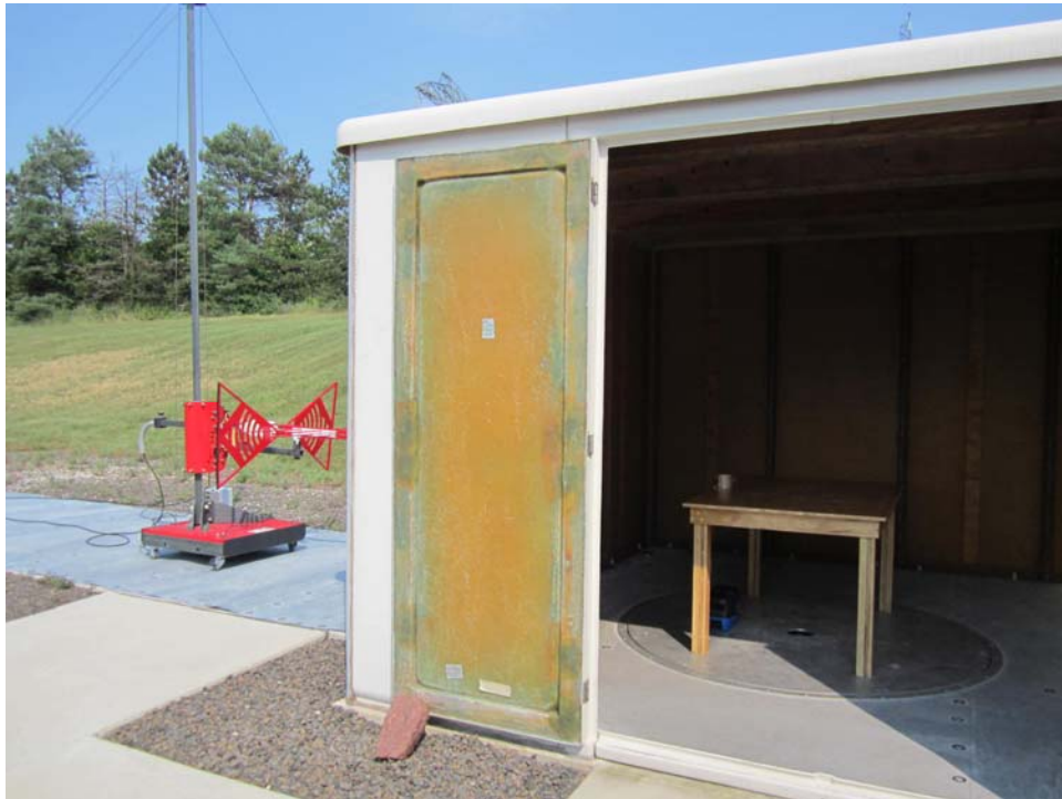
Horizontal Antenna Polarization
