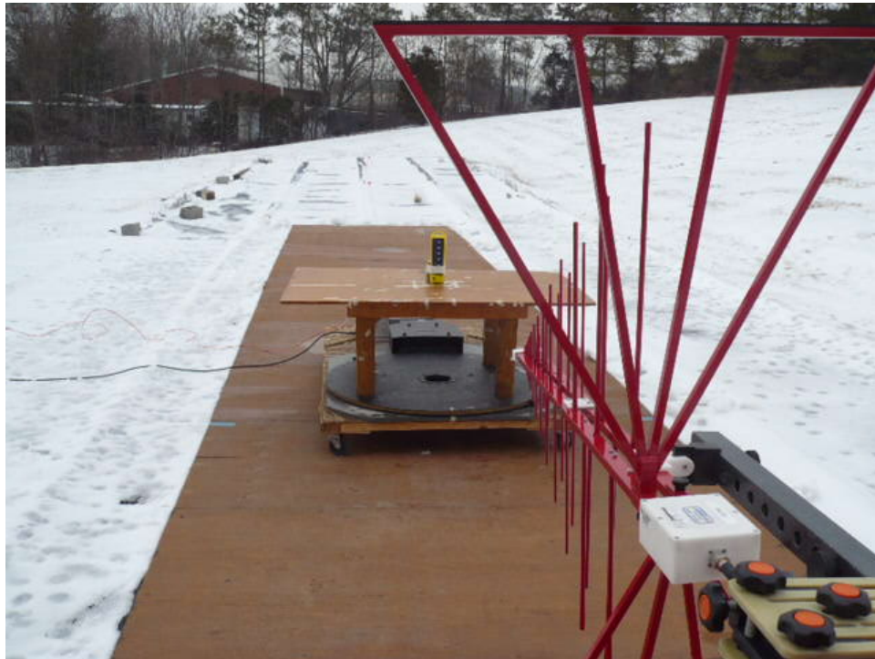
Biconilog Antenna, Vertical Polarization, 30 to 1000 MHz
