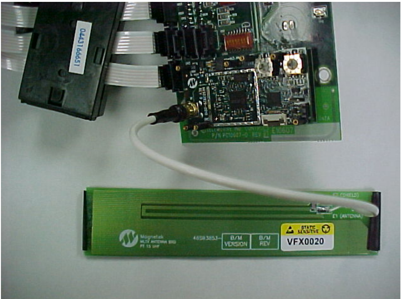
Photo Two – Internal RF Board/Top with Antenna/Bottom
