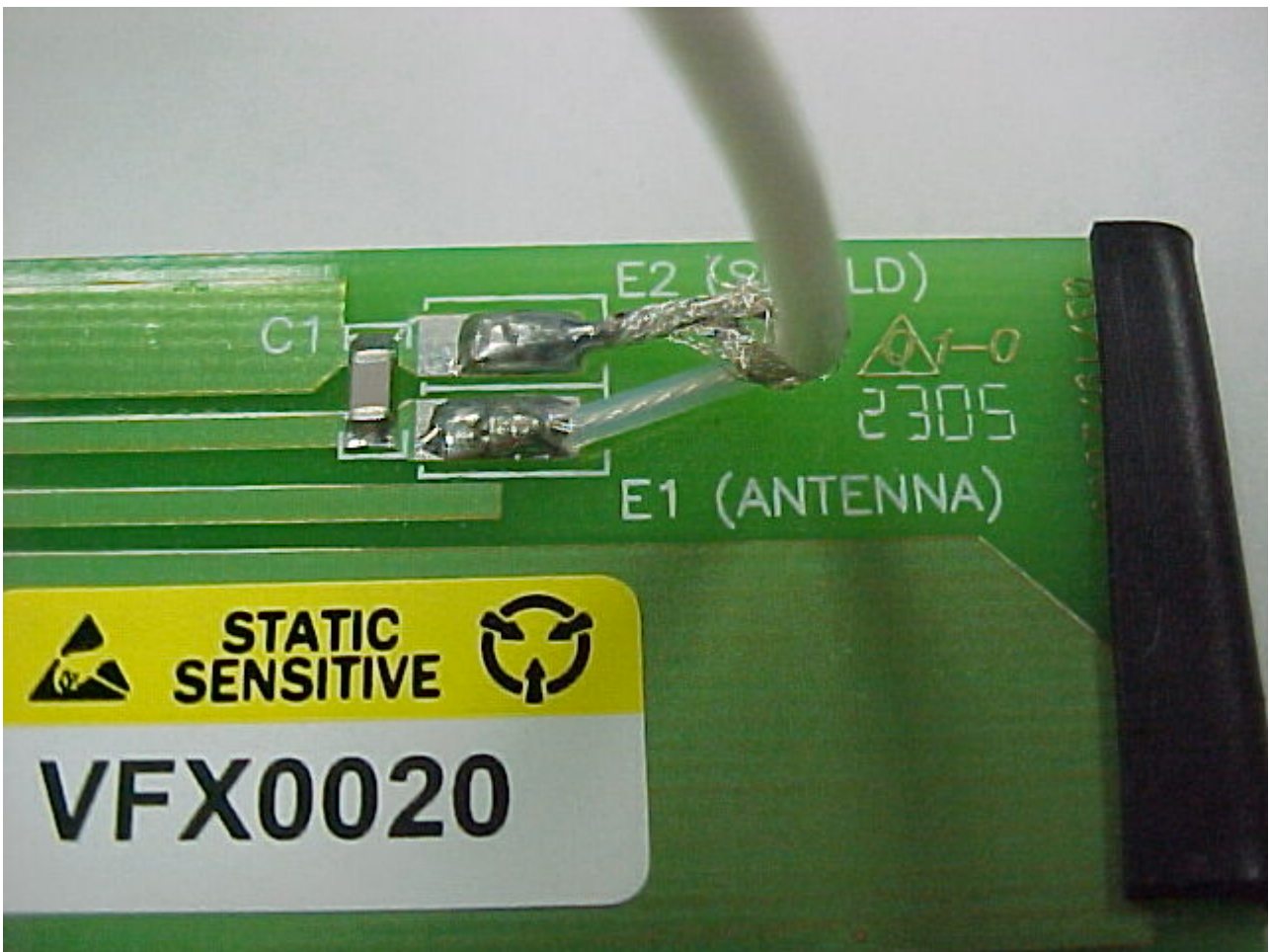
Photo Two – Internal Antenna Connection Close up
