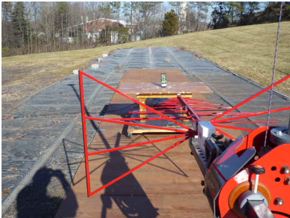
Biconilog Antenna, Horizontal Polarization, 30MHz to 1000MHz
