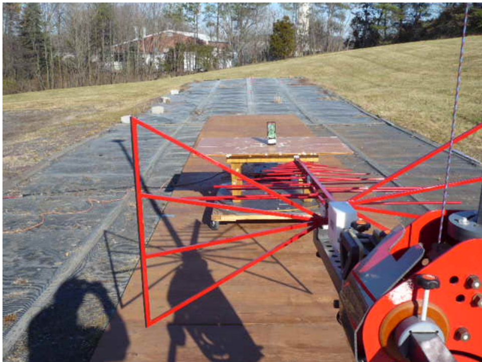
Biconilog Antenna, Horizontal Polarization, 30 MHz to 1000 MHz
