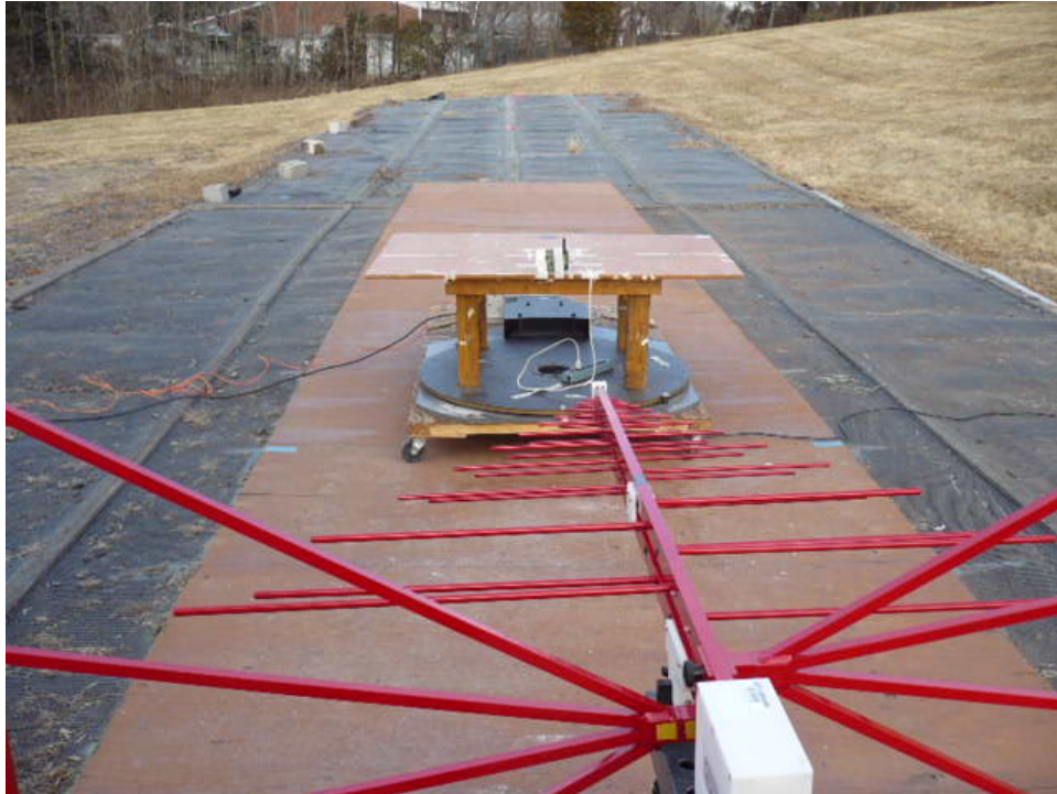
Biconilog Antenna, Horizontal Polarization, 30 MHz to 1000 MHz
