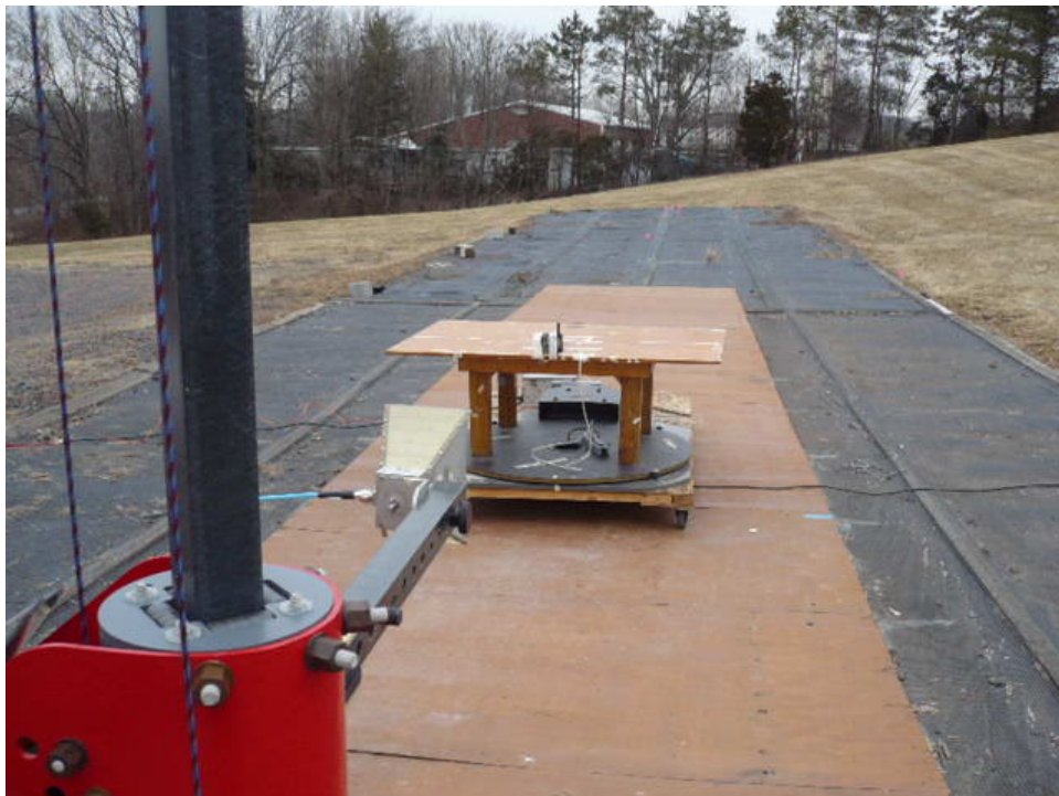
Double Ridged Guide, Vertical Polarization, 1 GHz to 18 GHz
