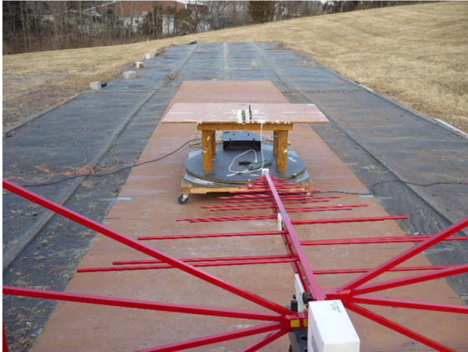
Biconilog Antenna, Horizontal Polarization, 30 MHz to 1000 MHz
