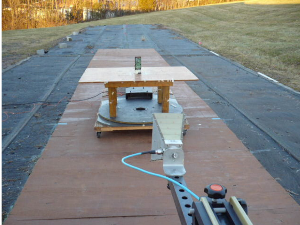
Double Ridged Guide, Vertical Polarization, 1 GHz to 4.4 GHz
