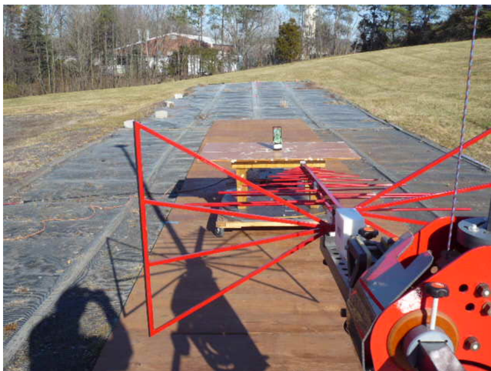
Biconilog Antenna, Horizontal Polarization, 30 MHz to 1000 MHz
