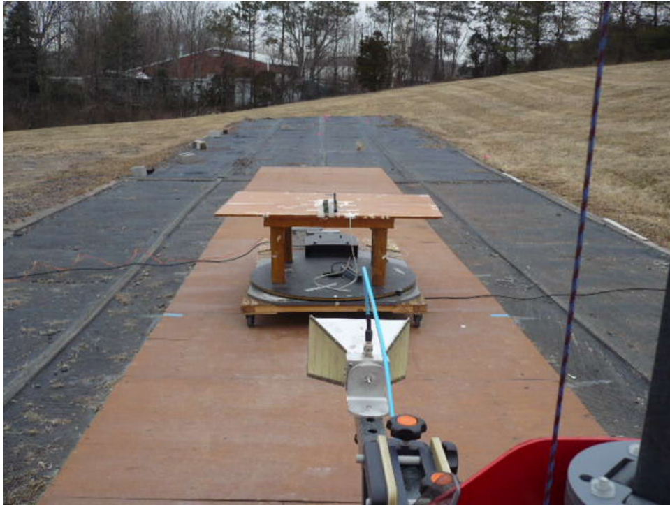
Double Ridged Guide, Horizontal Polarization, 1 GHz to 18 GHz
