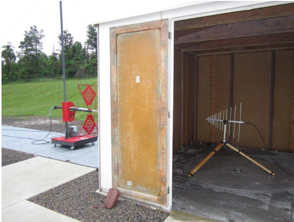
Biconilog Antenna, Vertical Polarization, Substitution Method
