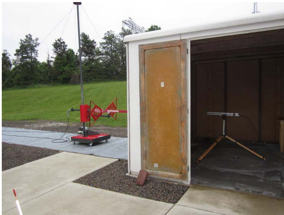
Biconilog Antenna, Horizontal Polarization, Substitution Method
