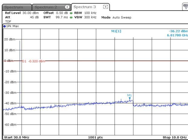
**Conducted spurious / Mid ch.**
