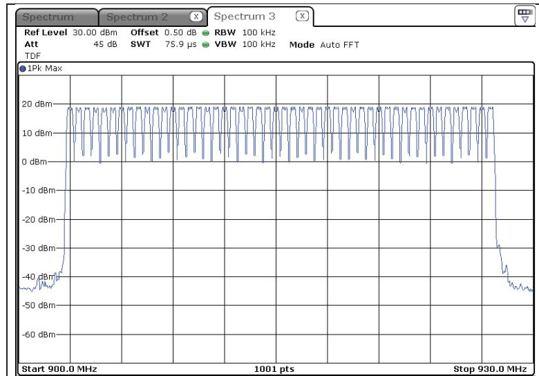
Figure 5. Plot of each individual hopping frequency sequence. (Conducted)
