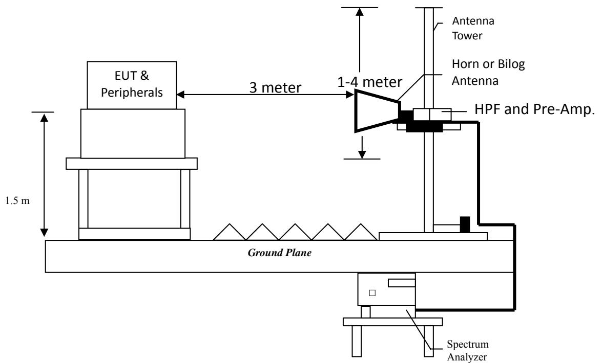
According to §15.33(a), the spectrum shall be investigated from the lowest radio frequency signal generated in the device, to the tenth harmonic of the highest fundamental frequency or to 40 GHz, whichever is lower. Spectrum Analyzer Resolution Bandwidth is 100kHz or greater for frequencies 30MHz to 1GHz, 1MHz – for frequencies above 1GHz.
