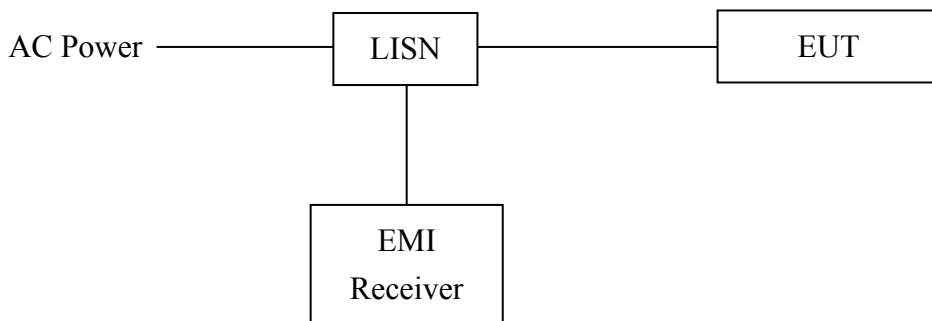
The test procedure was according to ANSI C63.10:2013.
