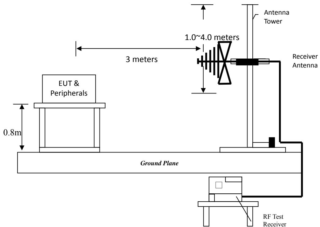
**Radiated emission above 1 GHz uses Horn Antenna:**
